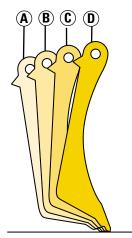
A 54° position offers maximum blade loads for production dozing, carry, backfill, and land clearing. Best position for finish grading.
